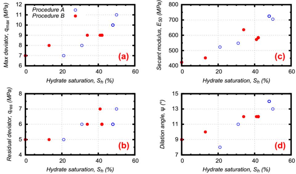
**Fig. 2: Sand's mechanical properties dependence on methane hydrate saturation for all tests**
