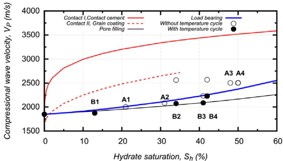
**Fig. 1: Comparison between experiments and Helgerud's model of compressional wave velocity dependence on methane hydrate saturation in water saturated media**
