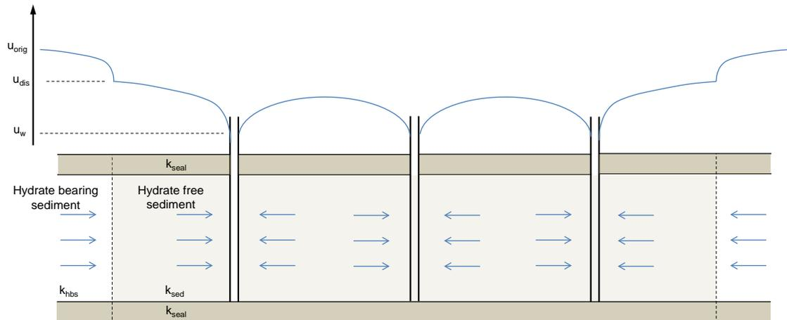
**Fig. 2: Multi well production strategy - Increased production volume. The design of the production system must take into consideration the pore water pressure at the well  $u_w$ , for dissociation  $u_{dis}$  and in the far field  $u_{orig}$ , and the permeabilities of the hydrate bearing sediment  $k_{hbs}$ , the hydrate-free sediment  $k_{sed}$ , and the seal layers  $k_{seal}$ .**
