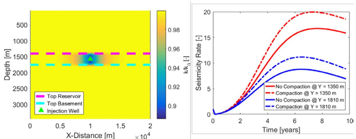
**Figure 1: An example result from a reverse faulting stress regime, (a) the permeability loss due to compaction and (b) the resulting seismicity rates when this permeability loss is and is not accounted for. The seismicity rates are taken at various depths (Y) vertically in-line with the producing well. The simulation is plane strain with injection occurring via a horizontal well.**
