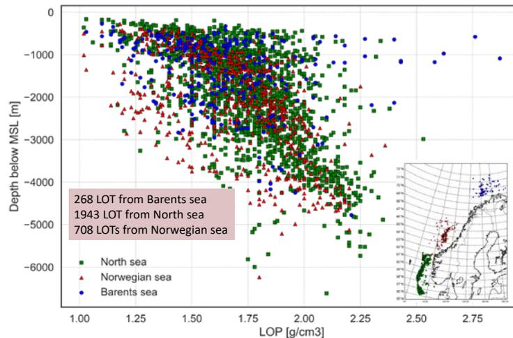
Fig. 1: Collected leak-off test data from NPD factpages (NPD, 2017).
