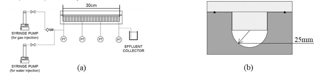
Fig. 1: (a) A schematic drawing of the 1-D flow test setup, and (b) the y-z sliced section of 1-D flow cell.
