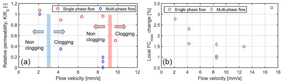
**Fig. 2: (a) Relative permeability changes during the single- and two-phase fluid flow, and (b) the maximum variation of local fines content measured after experiment.**
