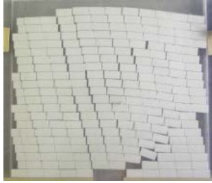
Fig. 2: a) Kinematic dilation of a laterally confined blocky medium with 90% inter-block overlap upon stimulation by imposing displacement on two blocks. b) Irreversible inter-block openings when the stimulation ceases
