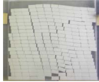
Fig. 2: a) Kinematic dilation of a laterally confined blocky medium with 90% inter-block overlap upon stimulation by imposing displacement on two blocks. b) Irreversible inter-block openings when the stimulation ceases
