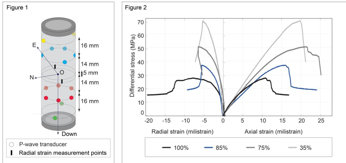
**Fig. 1: Position of the ultrasonic P-wave transducers on the cylindrical mudstone specimen**
