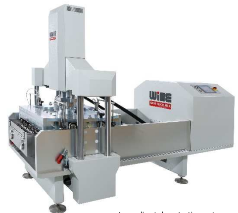
Large direct shear testing system
